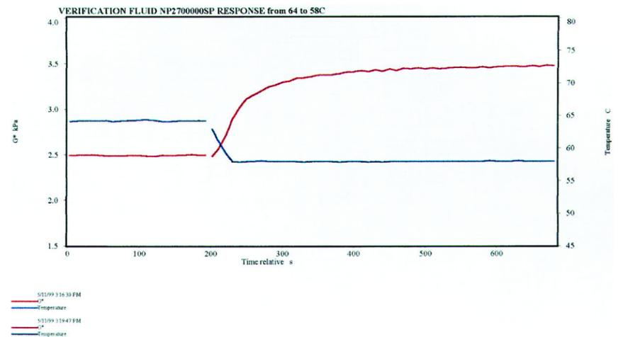
Figure 6 Temperature dependence of an original asphalt binder versus a calibration standard.
