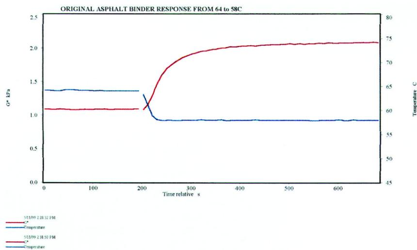
Figure 5 VISCOTECH DSR cooling transient response 64–58 °C.
