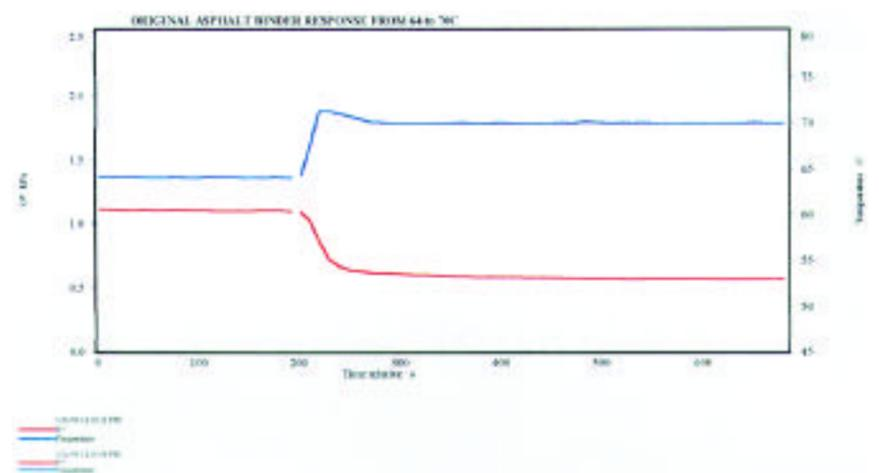
Figure 4 VISCOTECH DSR heating transient response  $64$ – $70^\circ\text{C}$ .
