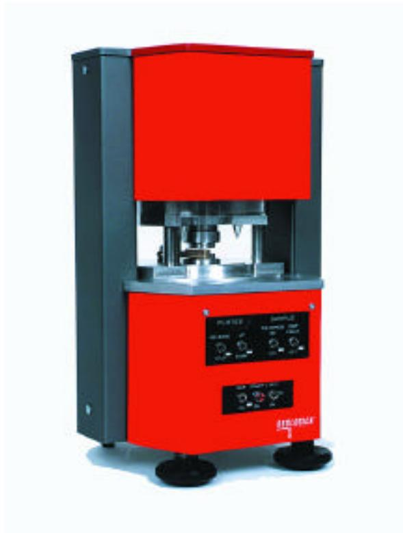
Figure 9 DSR QC dynamic shear rheometer.
