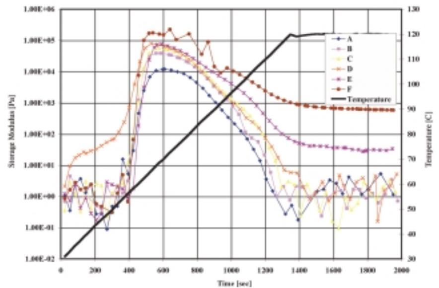
Figure 6 Storage modulus (Pa) and temperature (°C) plotted versus time (sec) for the six samples from the starch rheology experiment.
