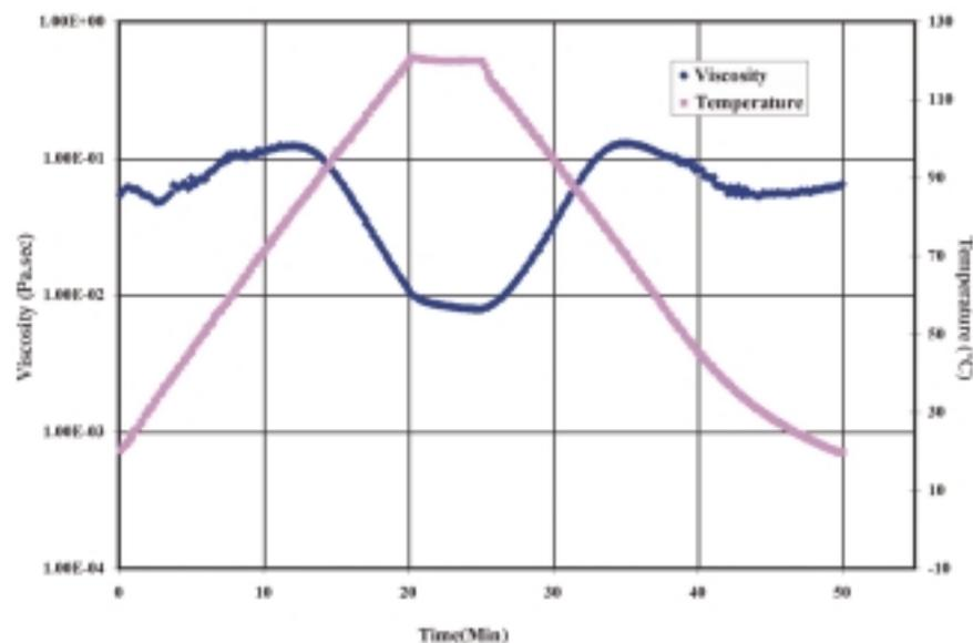
Figure 4 Gel from experiment in Figure 3 run under steady shear conditions with a temperature ramp back and forth from 20 to 120 °C at 2 °C/min at constant 100/sec.
