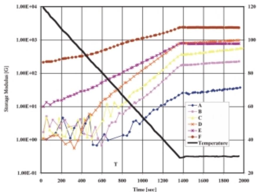
Figure 7 Linear viscoelastic properties of the gelatinized starch measured during a descending temperature ramp from 120 to 30 °C.
