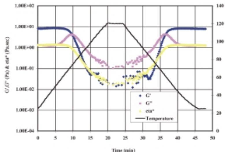
Figure 3 Results in the form of storage modulus ( $G'$ ), loss modulus ( $G''$ ), complex viscosity ( $\eta^*$ ), and temperature ( $^{\circ}\text{C}$ ) as a function of time for a dynamic experiment on a water-based gel using a 25-mm couette system.
