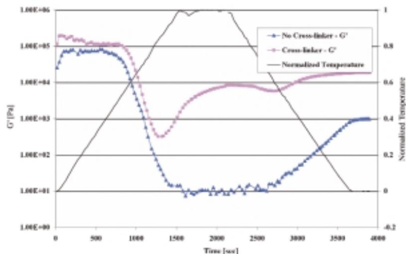
Figure 8 Cooking of mixtures of starch  $G'$  (see Table 1) and water with and without a cross-linking agent.
