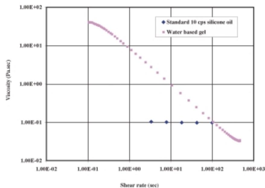
Figure 5 Shear rate sweep study performed on sample from experiment in Figure 3 at a constant temperature of 25 °C.
