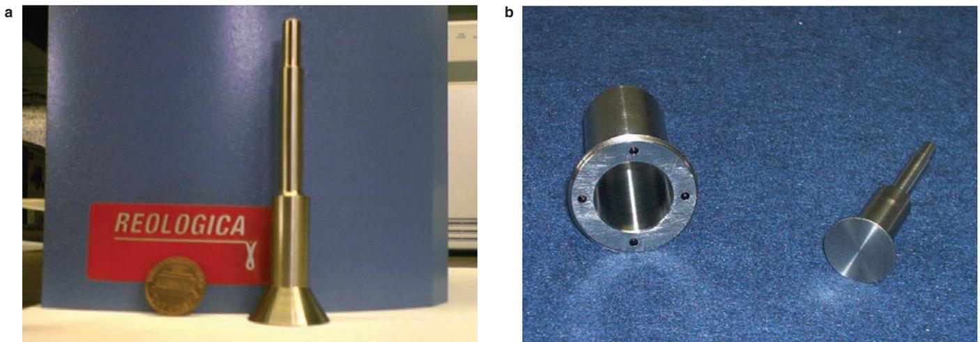
Figure 1 Friction Tool (25-mm) (a) and corresponding lower cup (b).
