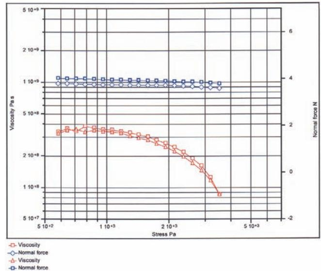
Figure 3 Viscosity (Pa s) and normal force (N) of sample A showing reproducibility.
