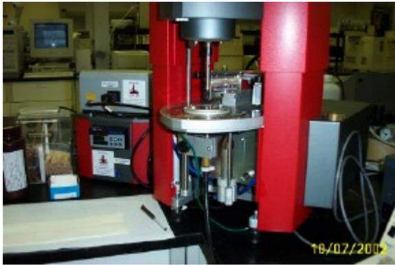
**Figure 1. StressTech Rheometer with UV Accessory.**
