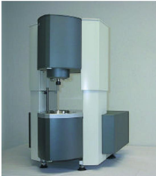
Figure 10 VISCOTECH rheometer.
