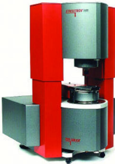
Figure 2 STRESSTECH HR rheometer.
