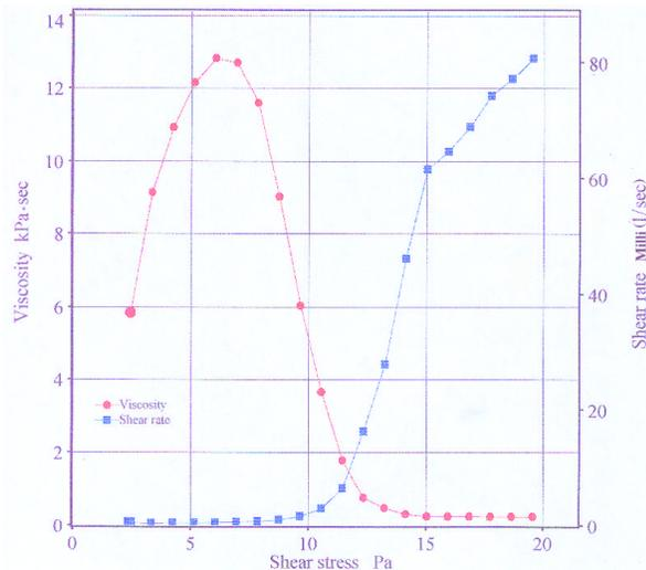
**Figure 2** Yield point determination in paint: CC 25; 2.000–20.00 Pa (up); 100.0 sec in 20 intervals; manual control; no. of measurements–1; measurement interval–50.0 sec; yield stress–6.047 Pa.
