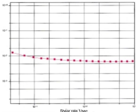
Figure 1 Graph of oil viscosity versus shear rate.
