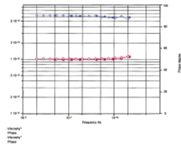
Figure 8 Frequency sweep complex viscosity versus frequency ambient and 300 psi pressure.
