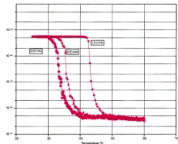
Figure 9 Oscillation temperature sweep complex viscosity versus temperature at three different heating rates: diamonds, 0.2 °C/min; triangles, 0.5 °C/min; circles, 1.0 °C/min.
