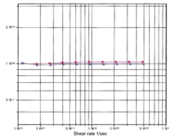
Figure 7 Flow curve viscosity versus shear rate oil, ambient (red circles), and 300 psi pressure (blue triangles).
