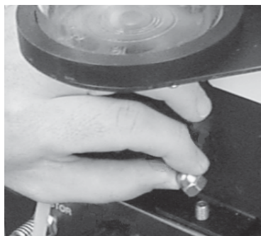
Figure 2: Securing the Bath Vessel Housing to the Control Chassis
