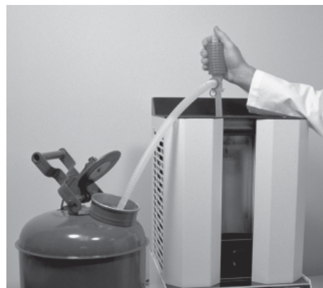
Figure 6: Removing fluid to a grounded metal waste receiver with a siphon
