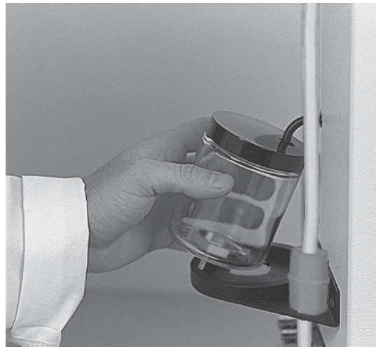
Figure 4: Overflow jar with platform and pump installed
