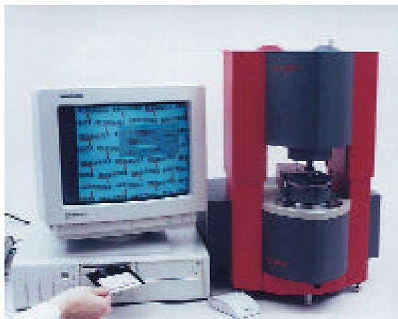
Figure 1 The STRESSTECH controlled stress/strain rheometer.
