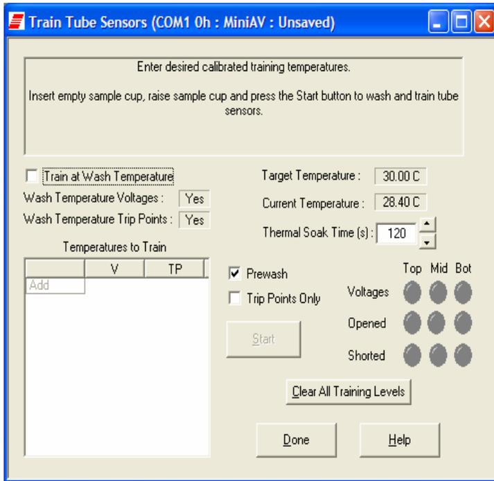
**NOTE:** *After the prewash is complete, the instrument will then obtain the voltages for each sensor at each of the specified temperatures.*
