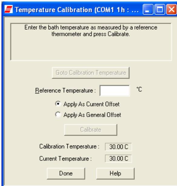
**NOTE: Occasionally a temperature may require several calibrations in order to get an accurate calibration**
