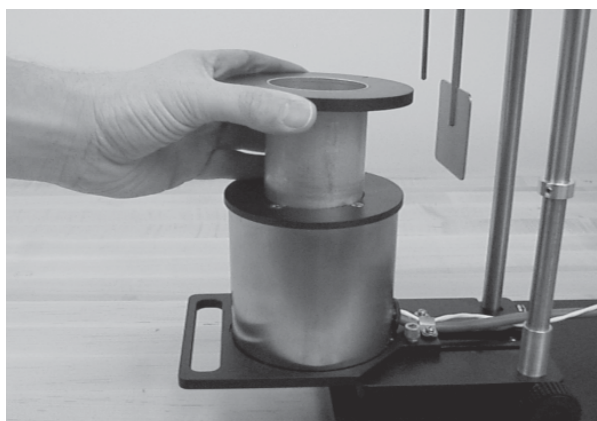
Figure 8: Inserting the sample cup into the heater block
