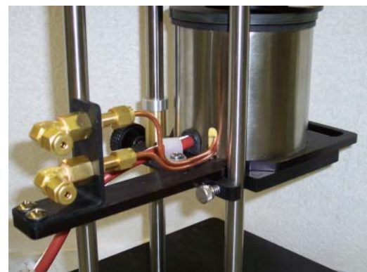
DPV with cooling coil option installed
