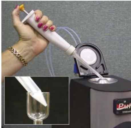
The **Ready to Test Screen** contains a **START** button. Pressing the button is optional as the injected sample will automatically be detected. The button is useful for higher viscosity fluids that may take a while to trip the top sensor.
