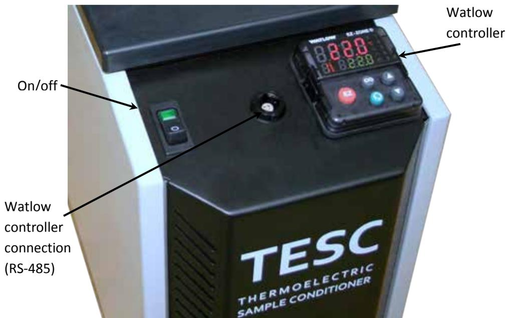
Figure 2 — TESC with Watlow controller
