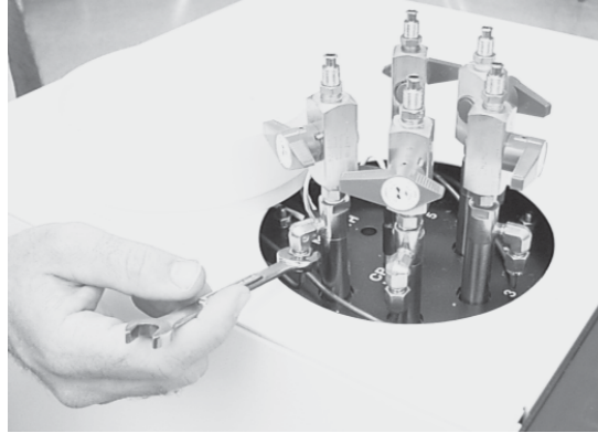
Disconnecting cell gas line connection
